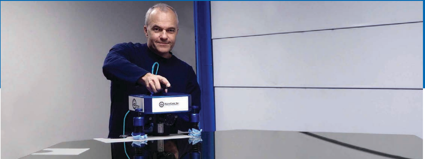
Vibration-insensitive NanoCam® Optical Profiler at Hawaii's Keck Observatory, shown here measuring a telescope mirror segment's finish. The portable profiler can be hand-placed or mounted to automation equipment for measuring complex objects with no contact.
