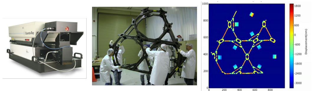
Figure 9. (left) Dynamic ESPI interferometer, (center) JWST backplane sample, (right) ESPI measurement of JWST backplane sample
