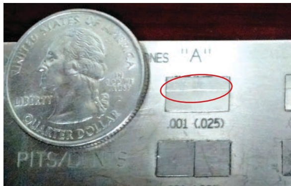
Figure 3: 0.001" scratch on visual comparison standard
