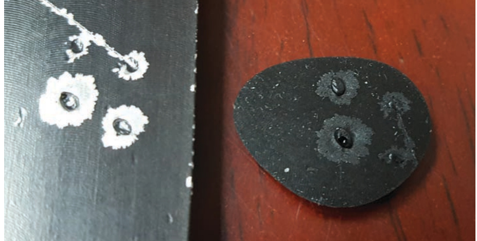
Figure 6: Pitted aluminum sample (left) and its replica (right).
