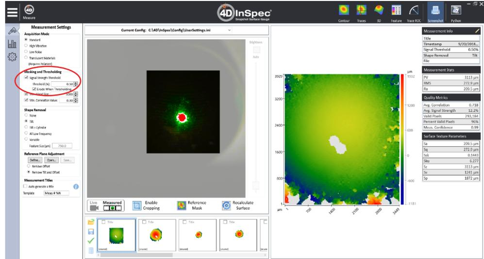
**Figure 5:** Data set of a ball bearing, using a signal strength threshold of 0.5% with cropping.
