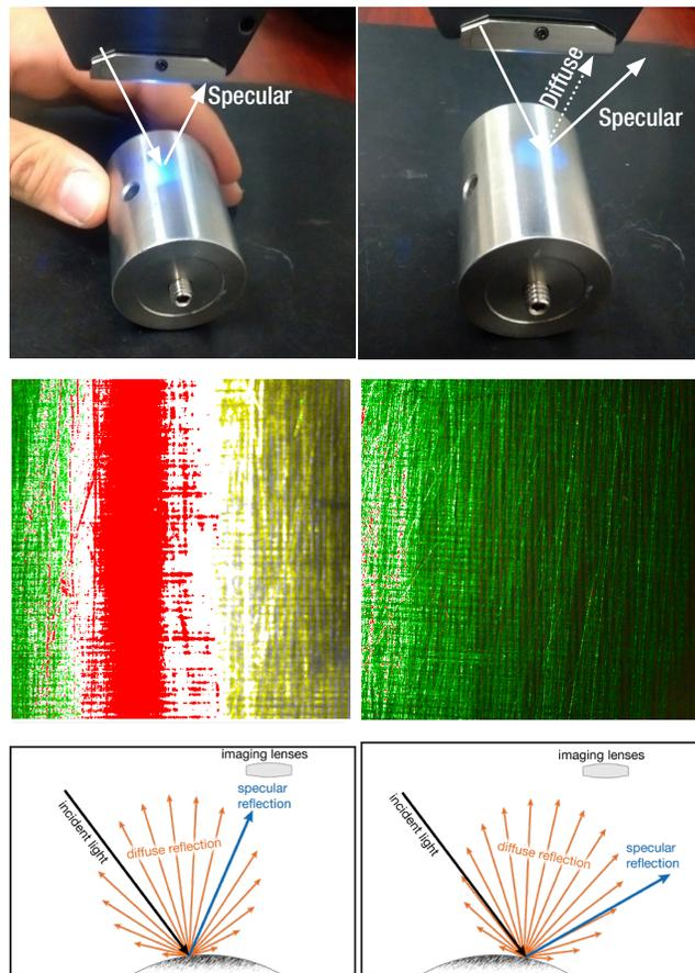
**Figure 3. Left** – An improper measurement angle results in saturation, shown as red pixels. **Right** – Shifting the cylinder (or angle the 4D InSpec) to illuminate a descending slope results in good data. 1
