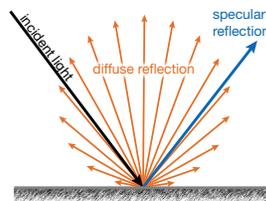
**Figure 1:** A beam of light's strong specular reflection leaves the surface at an equivalent angle to the beam's angle of incidence from the source. Surface irregularities scatter light from the illuminated area in a diffuse reflection.<sup>1</sup>
