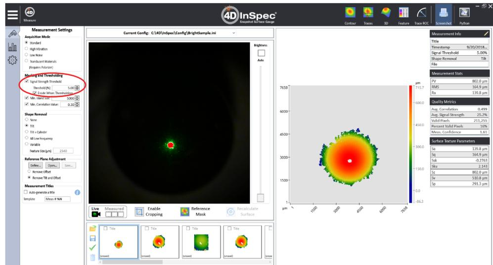
**Figure 6:** Data set from the same ball bearing as figure 4, but with a higher signal strength threshold of 5%.
