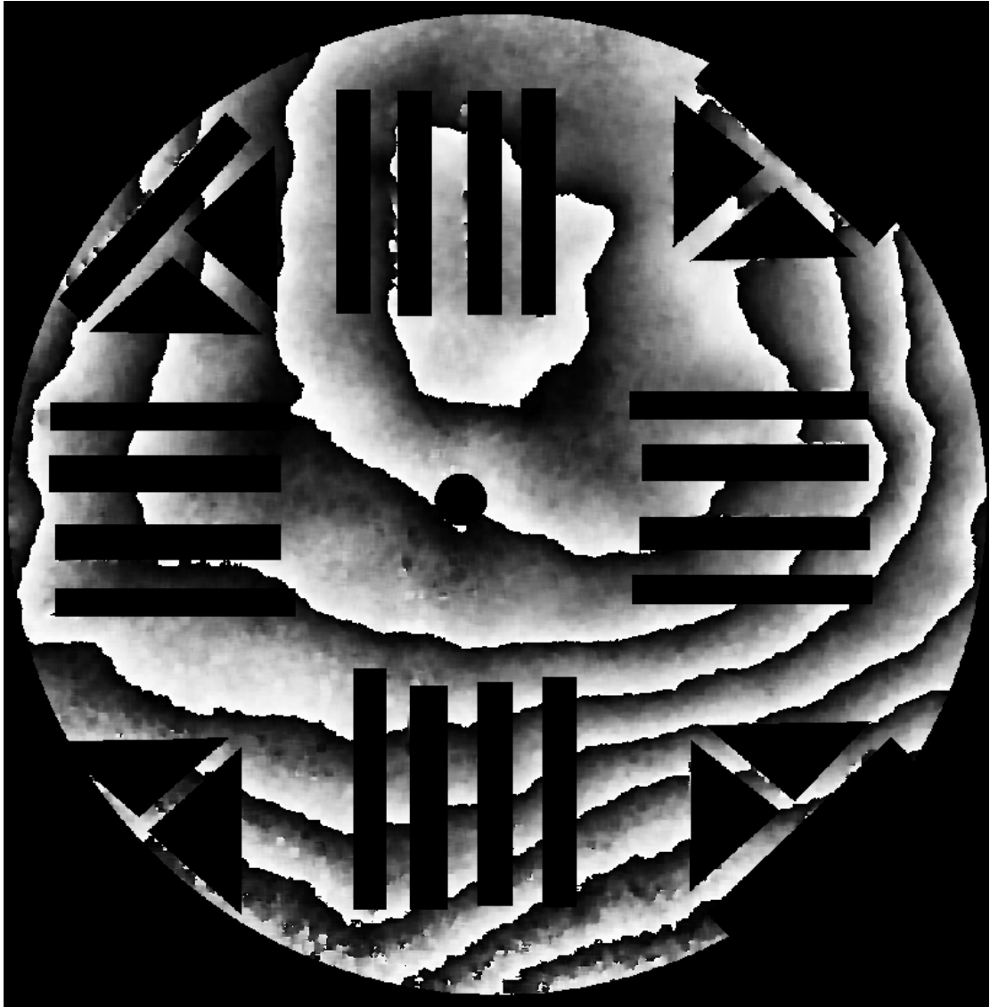
Figure 4: Wrapped phase from measurement of a 1m carbon fiber target
