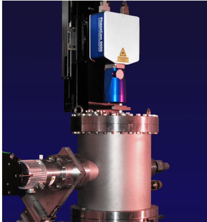
PhaseCam Twyman-Green interferometers measuring into an environmental test chamber (Courtesy CNRI)
