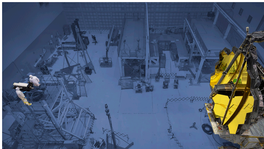
PhaseCam completing Center of Curvature test for the Webb Space Telescope (courtesy NASA Goddard)
