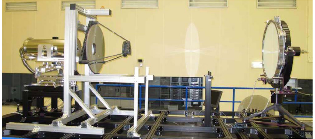
Vacuum-compatible PhaseCam inside a large vacuum chamber (courtesy JAXA)
